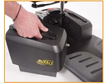
Step 2: Pull out the battery pack!
