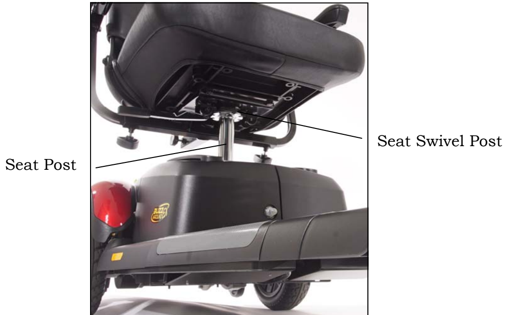
Figure 23. Installing the Seat
