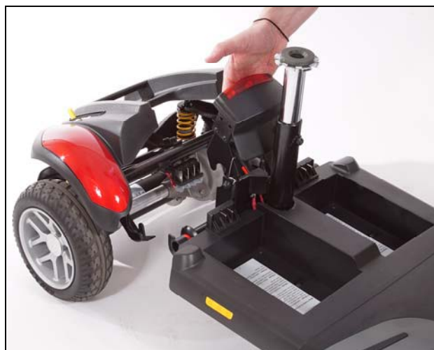
Figure 17. Separating the Drivetrain and Frame
