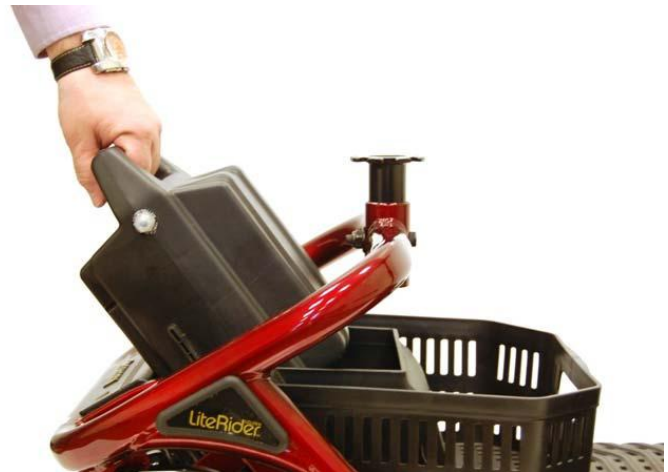
Figure 21. Battery Pack Installation
