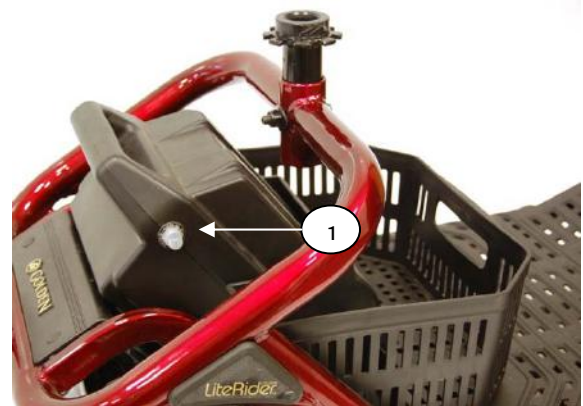
Figure 27. Main Circuit Breaker
