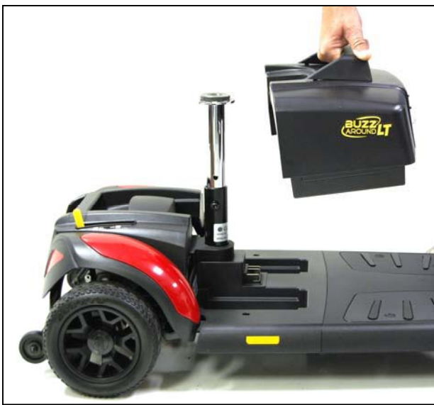
Figure 21. Battery Pack Installation
