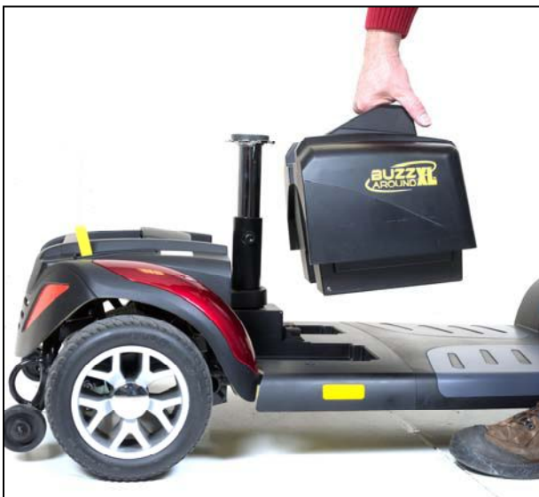
Figure 21. Battery Pack Installation
