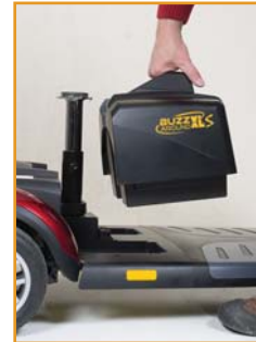
Step 2: Pull out the battery pack!
