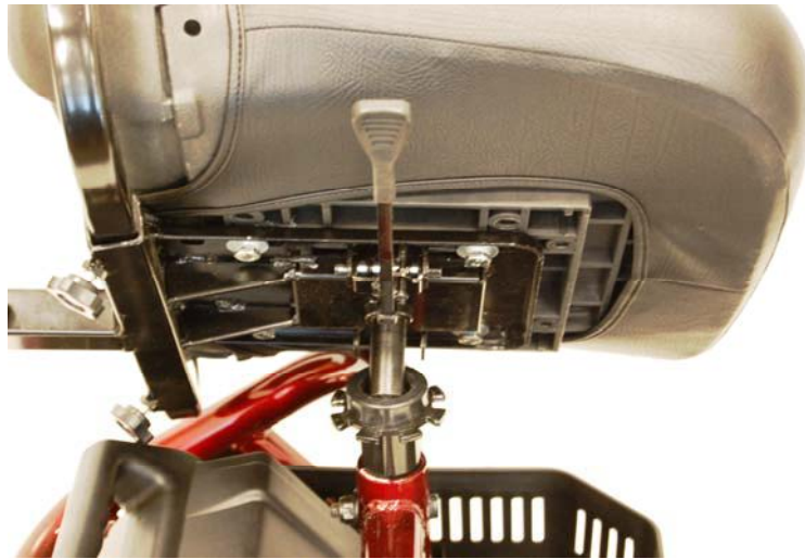
Figure 23. Installing the Seat
