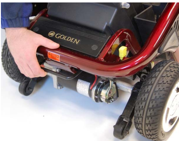
Figure 17. Releasing the Drivetrain
