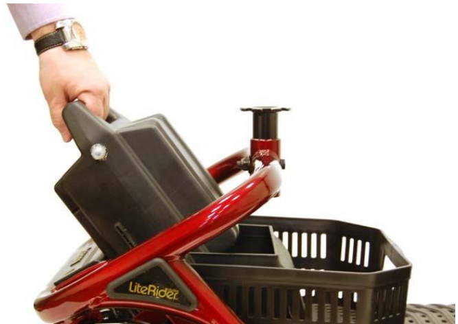
Figure 21. Battery Pack Installation
