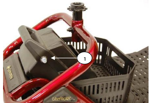
Figure 27. Main Circuit Breaker
