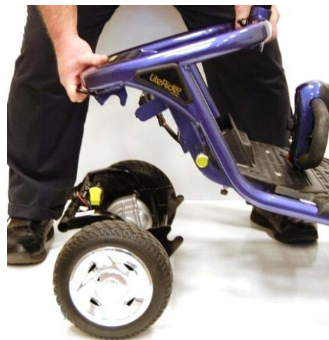
Figure 18. Lifting the Frame
