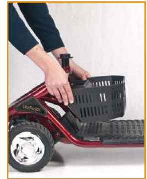
Remove the baskets from under the seat and from the tiller (not shown)
