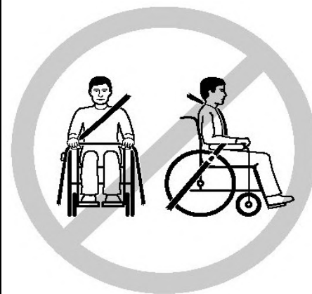
Incorrect seat belt position
