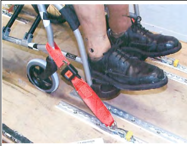
Fitting the front restraint
