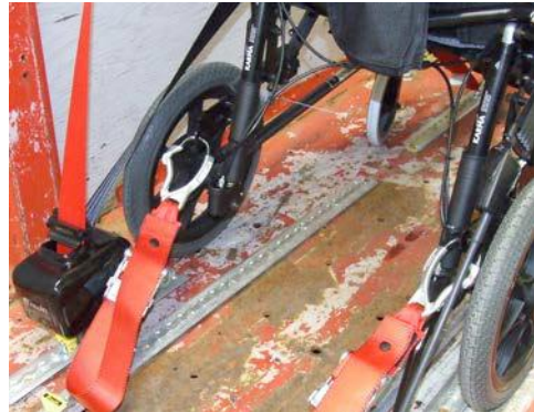
Fitting the rear restraint
