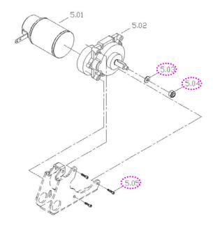
Replace the driver wheel by the following steps if it is worn out or deformed.
