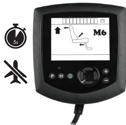
Figure 111. Give and hold a forward command for 5 seconds. Airplane mode is off.
