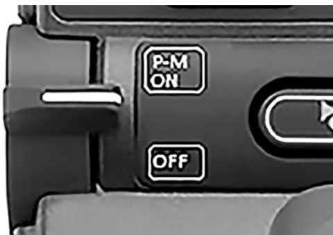
Figure 16. Power, mode and profile paddle.
