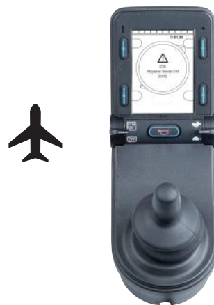
Figure 105. Airplane mode is on.
