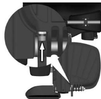
Figure 138. Adjusting the footplate angle
