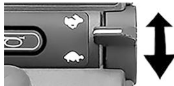
Figure 50. In mode Bluetooth® the right paddle switch is used to scroll up or down.
