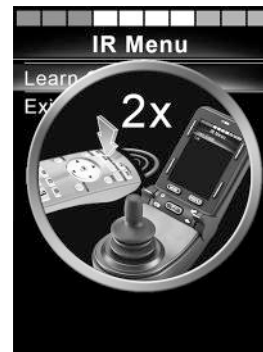
Figure 58. Point the remote control at the IR receiver. Press the button twice.
