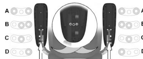
Figure 131. Adjusting the armrest swivel end position.
