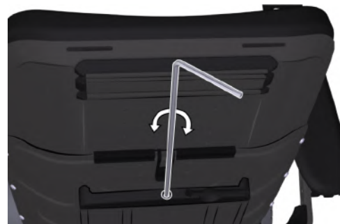
Figure 134. Use the supplied adjustment crank.
