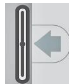
Figure 22. Left turn signal button and screen symbol.
