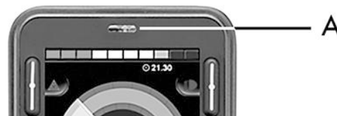
Figure 54. The IR receiver location.
