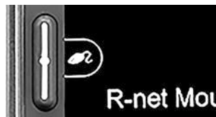
Figure 48. Left button for left mouse clicks.
