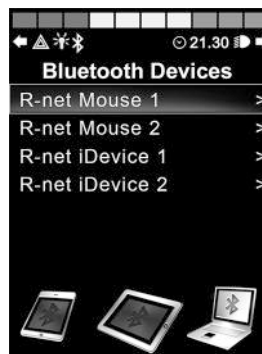
Figure 43. The Bluetooth® Device screen from which paired devices are chosen.
