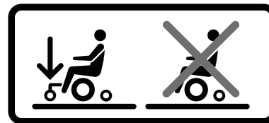
Figure 116. The support wheels must always be fitted when you drive.
