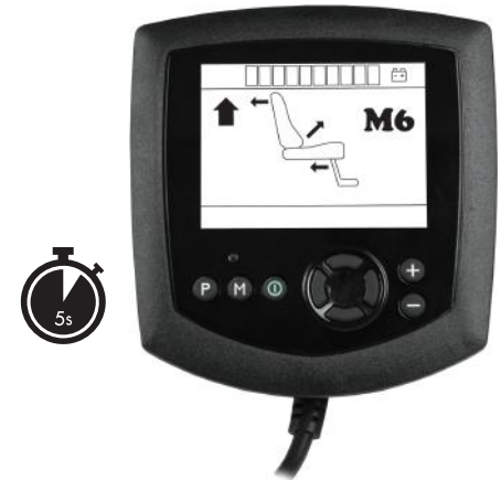
Figure 106. Give and hold a forward command for 5 seconds.
