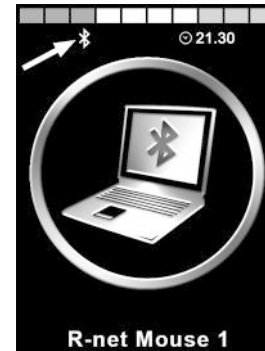
Figure 41. The arrow points to the flashing Bluetooth® icon.
