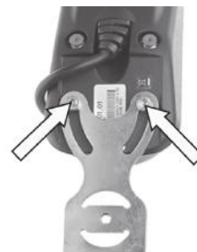
Figure 144. Only remove one of the screws.
