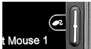
Figure 49. Right button for right mouse clicks.
