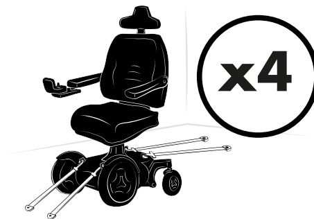
Figure 165. The wheelchair has four tie-down points. The wheelchair and tie-down position in this picture is generic.
