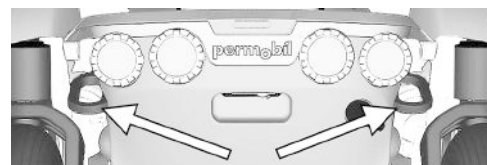
Figure 1 67. Rear tie-down eyes.
