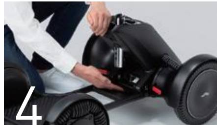
Pull the lever on the side of the battery toward you to separate the parts.
